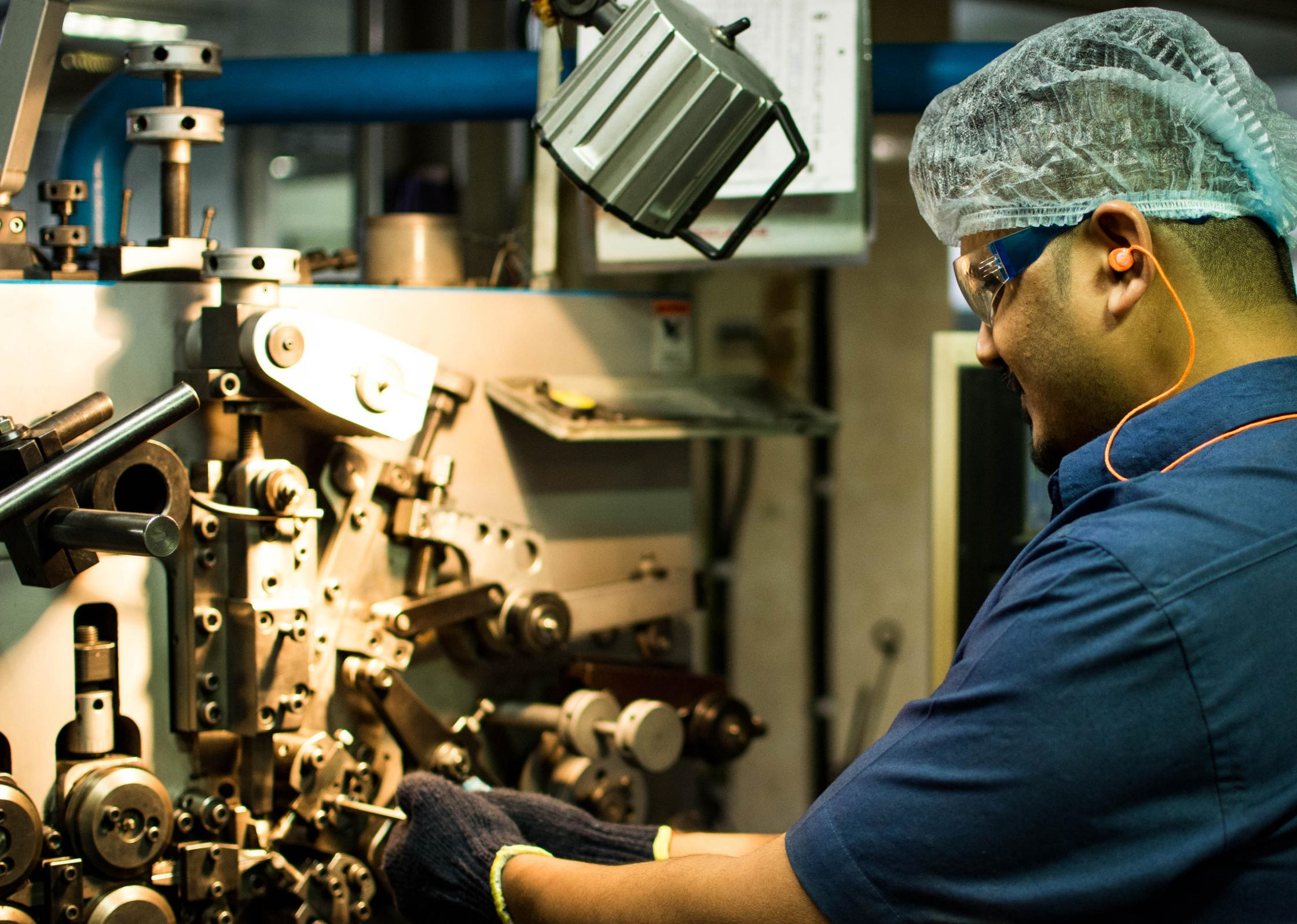
After obtaining a spring from the CNC machine in case of compression springs, they undergo the process of heating and grinding.
