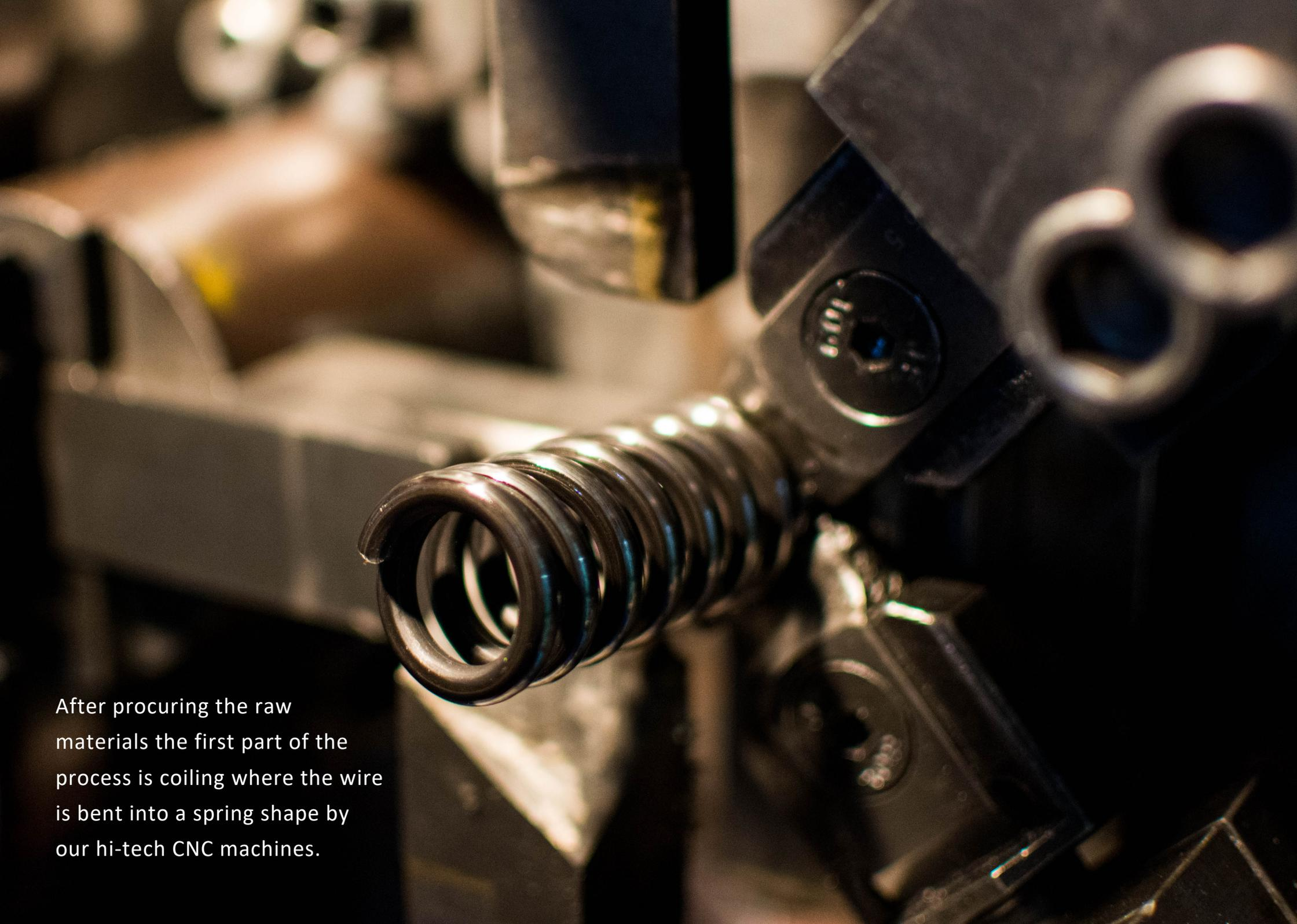
After procuring the raw materials the first part of the process is coiling where the wire is bent into a spring shape by our hi-tech CNC machines.
